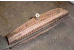
Apply epoxy as before and use the vise to press the pins home. DO NOT try too hard. The hole will have a bevel at the bottom due to the shape of the drill, so the pins may be 1/16 to 1/8" long. Once the majority is in the handle, you're done. Trying to push the pins through what remains of the wood in line with the hole and the hardened tang is NOT a good idea.
