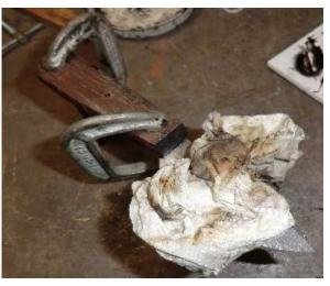
After the glue has set (it takes 24 hours to reach max strength but 10 to 15 minutes to stop sticking to you when you touch it), you can go back to the drill press and drill the remaining pin holes (tang side up, of course). If you are excessively anal about tight clearances for the pins, use a slightly smaller drill bit to drill the holes. Remember what was said about the center line of the tang being the reference plane.
