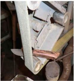
Once the grinding is done, it's over to the buffer. I usually hit the handle with white rouge on a muslin buff. It's a good idea to go lightly on the mosaic pins. After that, the tape is removed and the knife is hit with a degreaser/cleaner (like 409) and a scrub down with an old tooth brush. This ought to remove any polish and adhesive left on the knife.
