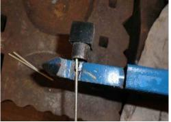
The pins have a pointy end and are of varying lengths. Match the pins to the width of the handles at the various hole locations and tap (NOT drive - TAP) them in pointy end first. It is easy to split slabs by driving a pin at an angle to the hole. It is easy to pop a slab free if the pin hits the tang rather than passing through it. This is why the tang holes are oversized and chamfered and the pins are pointed.
