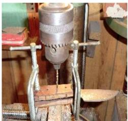
Just as for the 1st slab, it helps to assemble the clamps, alignment pin, and components that are to be glued before mixing the epoxy. As with the first slab, it really doesn't matter which side the alignment pin is inserted from, just so long as it extends far enough to "catch" the other side.
