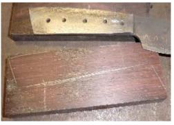
Saw the pieces out -- and saw outside of the lines. It's easy to grind away excess wood and a pain if you have to grind away part of the steel and/or start over because you cut into the tang's outline. I find that having a desk lamp positioned at the band saw makes this operation a lot nicer.
