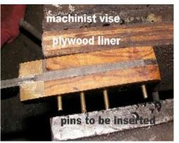
Depending on the amount of bulge in the handle (if any), you might have to individually press the first and last pin as shown. Another way to avoid this problem is insert the pins before shaping the handle. The advantages are all pins are the same length and the probability of watching the slabs fall off is lower (but if you overheat the epoxy, it will be compromised). The downside is more pin stock used.
