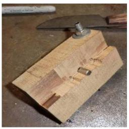
the block is placed on a vertical metal cutting band saw (the cheap one from Harbor Freight works). The blade positioned in the top-to-bottom slit, the stock extending to the right is in your right hand, and (with both hands) the block is slid forward to cut the pin stock. Once the cut is made, the bolt is slackened, the pin section pushed out of the hole, and the one end if the section is beveled on the grinder.
