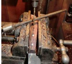
You can now switch out the small drill bit for the one to be used with the mosaic pins. Drill the hole. DO NOT attempt to drill through the tang. Go in at least 0.25" but stop when you feel or hear the tip hitting the tang. The tang is probably hard and all you will do by attempting to drill through it is to compromise the epoxy and potentially destroy the handle.
