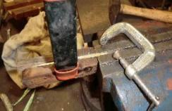
In this image, there is one clamp positioned at the tail and another at the head of the handle. Once they are in place, the spring clamp can be removed, the knife removed from the vise, and it's time to go to the drill press again.
