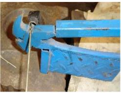
and then flies across the shop. To prevent that, a magnet from a hard disk is positioned on the farside of the shear and a capped section of light steel pipe is placed on the magnet. When the material is sheared, the pin now ends up in the cup. I figure the time spend chasing down flying pins is far greater than the fabrication time for this tool.
