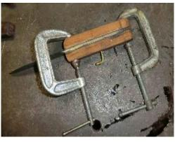
Follow the procedure outline above and epoxy the remaining slab to the knife. Make sure to match the outline, to secure the clamps and to clean the interface and blade of any excess epoxy.
