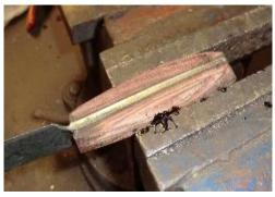
You now have something like the condition of the pins after epoxying. Back to the grinder and grind the pins flush to the surface of the handle. If you haven't already shaped the handle, do that now.
