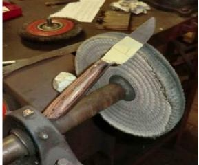
If we are talking Damascus, the knife is hit with gun bluing - not just the blade but the exposed metal of the tang. It is then wet sanded using 2000 grit paper.
