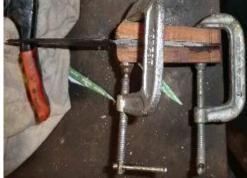
You can now drill through the existing holes to complete the holes in the handle. If you have used an undersized drill bit, this is when you drill using the bit matching the pins and/or use a reamer.
