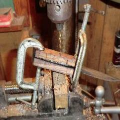
Assuming that you get the clamps positioned correct way up, you can now drill through the hole that once held the alignment pin, through the tang and through the 2nd slab. Note that if you are using C-clamps and the length of the handle is a bit short, there may be issues with the drill press chuck hitting the clamps.
